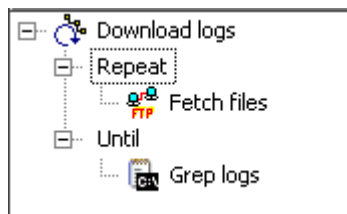
Download files from an FTP server until one of them contains a particular string we are looking for. The moment the string is found we end execution.
